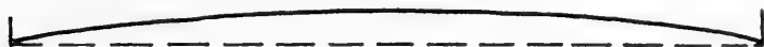
FIG. 225.—Showing proper curvature of finished roadway so as to insure good drainage.
